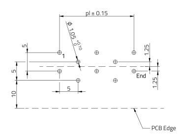
Recommended PCB Thickness : 1.6mm
