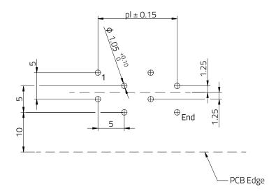
Recommended PCB Thickness : 1.6 mm
