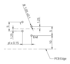
Recommended PCB Thickness: 1.6 mm
