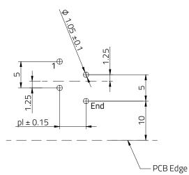
Recommended PCB Thickness : 1.6 mm
