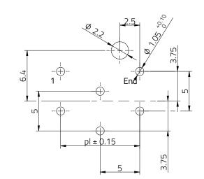
Recommended PCB Thickness : 1.6mm
