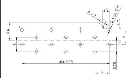
Recommended PCB Thickness: 1.6mm
