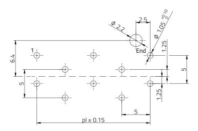
Recommended PCB Thickness: 1.6mm
