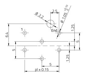
Recommended PCB Thickness: 1.6mm
