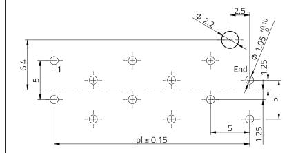
Recommended PCB Thickness: 1.6mm
