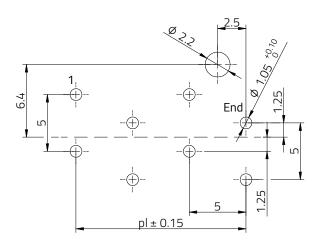
Recommended PCB Thickness: 1.6mm
