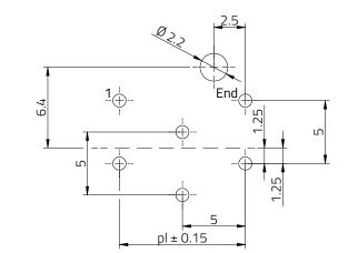
Recommended PCB Thickness : 1.6mm
