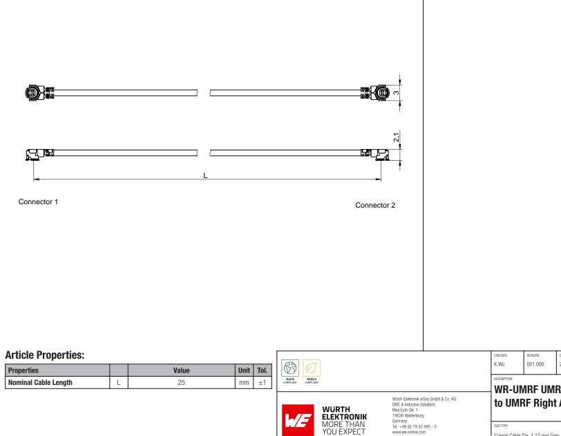
DATE (YYYY-MM-DD) GENERAL TOLERANCE PROJECTION METHOD 2022-09-14 DIN ISO 2768-1m **WR-UMRF UMRF Right Angle Plug** to UMRF Right Angle Plug ORDER CODE 636201050025 STATUS BUSINESS UNIT PAGE Coaxial Cable Dia. 1.13 mm Grey Jacket eiCan Valid 1/6
