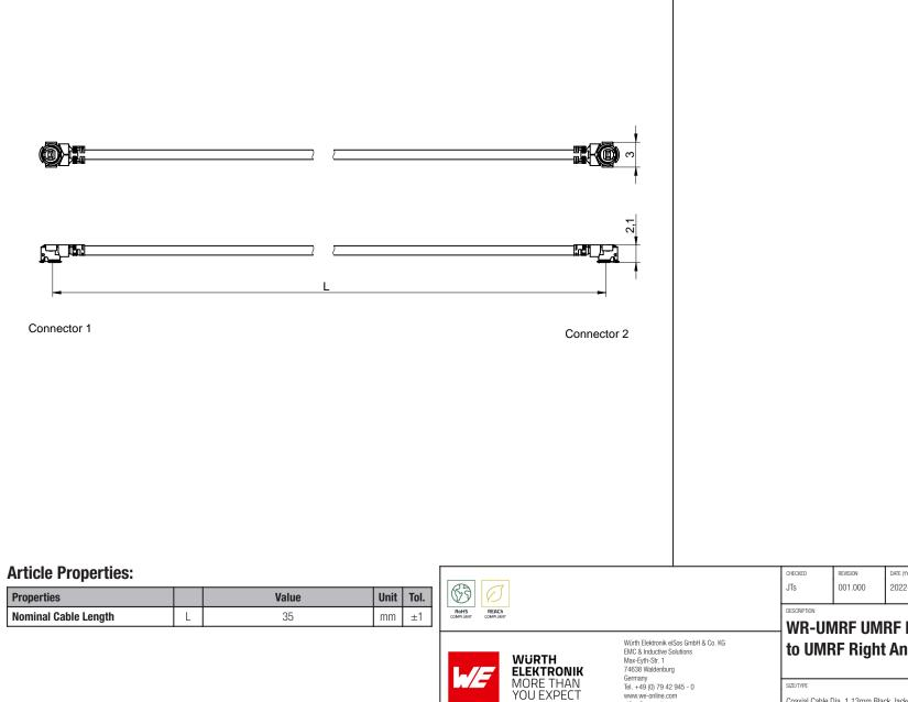
DATE (YYYY-MM-DD) GENERAL TOLERANCE PROJECTION METHOD 2022-05-05 DIN ISO 2768-1m **WR-UMRF UMRF Right Angle Plug** to UMRF Right Angle Plug ORDER CODE 636201040035 STATUS BUSINESS UNIT PAGE Coaxial Cable Dia. 1.13mm Black Jacke eiCan Valid 1/6
