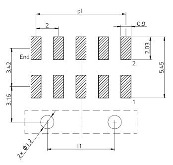
Recommended PCB Layout General tolerance ±0.05
