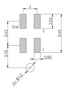
Recommended PCB Layout General tolerance ±0.05
