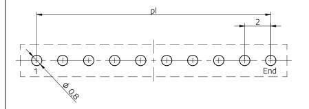
Recommended PCB Layout General tolerance ±0.05
