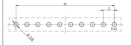
Recommended PCB Layout General tolerance ±0.05
