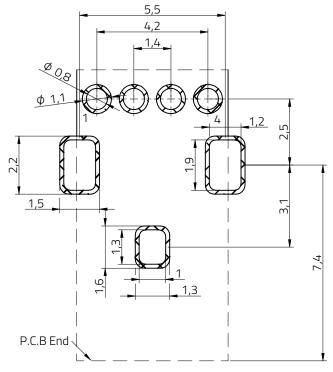
General tolerance ± 0.05 Recommended PCB Thickness : 1.20 mm ± 0.05
