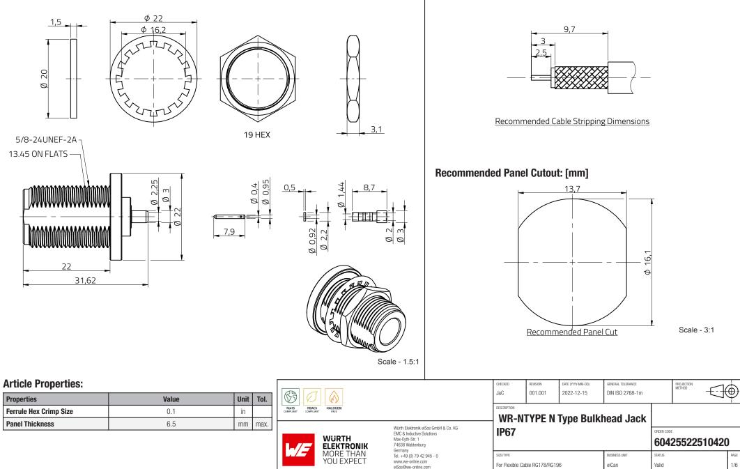
**Recommended Cable Stripping Dimension: [mm]**
