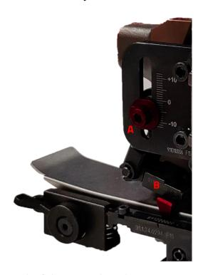
For adapting the pawl B to the pitch of the terminals, to have a new terminal correctly placed on the anvil for each cycle of the press: loosen the nut A and move the screw up for a greater pitch or down for a shorter one. Then tighten the nut again.
