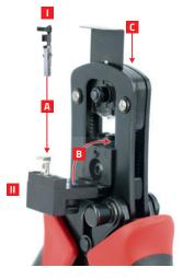
Insert the correctly stripped cable into the contact until the wire hit the wire stop (D).
