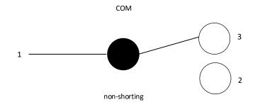
Type of Schematic: SPDT
