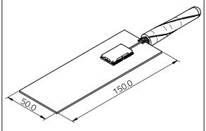
The 50 x 150 mm surface is a ground plane, which is not included with the antenna. Scale - 1:2,5
