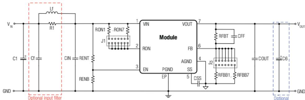
The additional aluminium electrolytic capacitor C1 is only for evaluation board protection purposes. It is mounted at the termination of the supply line and provides slight damping of possible oscillations of the series resonance circuit represented by the inductance of the supply line and the input capacitance. It is not essential for operation. The switching frequency of the module can be adjusted by changing the position of jumper J1.
