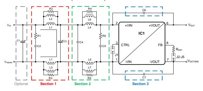
The VISM evaluation board is a multi-functional EMI optimization tool. It offers the possibility to optimize the EMI behavior based on the application requirements by placing multiple differential (DM) and/or common mode (CM) filters. Therefore the evaluation board consists of three different filter sections. The tables below show the main component selection possibilities:
