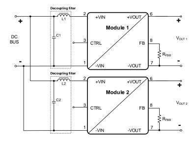
As a starting point for the decoupling filters, use the values of the reference filters – see also "<u>RADIATED AND CONDUCTED</u> <u>EMISSIONS (WITH EMI INPUT FILTER)</u>". The final appropriate filter for the application has then to be evaluated under operation in the target application by checking e.g. the change of the input ripple voltage.
