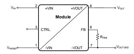
The output voltage is determined by the value of the external feedback resistor and the internal feedback resistor which create a voltage dividing network within the module. The output voltage adjustment range is from 3.3V to 6V. The ratio of the feedback resistors for the desired output voltage is:
