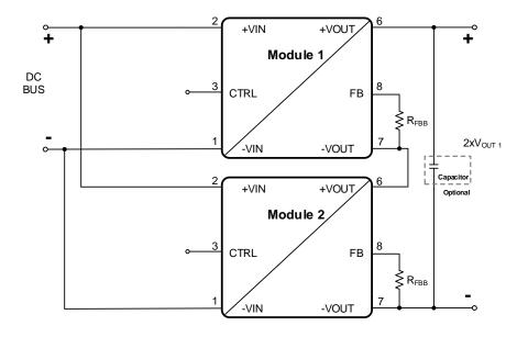
In case of using long supply lines or different line length for each 17791063215 it is recommended to decouple each power module with an additional LC filter. The decoupling LC filter is also recommended if the suppling dc bus has a high impedance so that high voltage swings at the input of each power module could be present. See also "Primary side parallel connection" on page 25.
