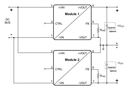
For using long supply lines or different line length for each 17791063215 it is recommended to decouple each power module with an additional LC- filter. The decoupling LC-filter is also recommended if the suppling dc bus has a high impedance so that high voltage swings at the input of each power module could be present. See also "Primary side parallel connection" on page 25.
