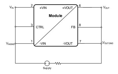
Parameters Supply Device: Current limit set 500µA, test voltage 2000Vdc, test time 60sec.
