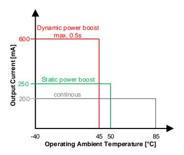
**Note:** Power Boost available for  $V_{IN}=8V$  to 36V  $V_{OUT}=5V$ ; still air (0-20LFM/0-0.1m/s)
