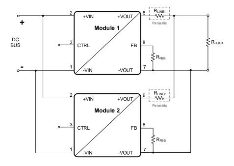
In case of using long supply lines or different line length for each 17791063215 it is recommended to decouple each power module with an additional LC filter. The decoupling LC filter is also recommended if the suppling dc bus has a high impedance so that high voltage swings at the input of each power module could be present. See also "Primary side parallel connection" on page 25.
