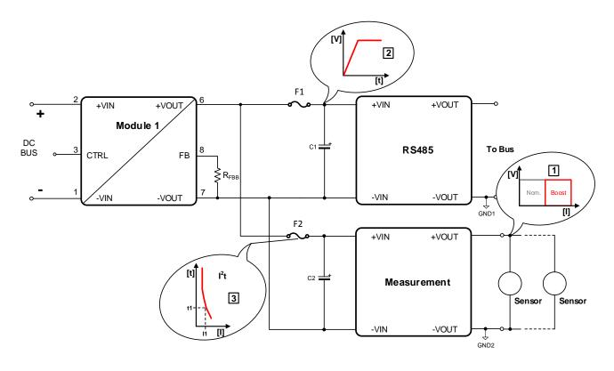
The power boost feature provides additional current, allowing the module to fulfill the following demands:
