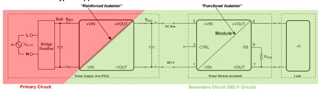
The 177 910 63215 Magl<sup>3</sup>C power module is only intended to be used as a CLASS III equipment according to the UL60950-1 & UL62368-1 standard. That requires that the power module is supplied by a **SELV** (safety extra low voltage) or ES1 circuit which provides protection against electric shock. There are no HAZARDOUS voltages present in CLASS III equipment.
