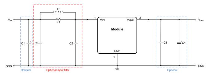
The 173950x78 integrates both the input and output capacitors. Therefore, additional external input/output capacitors are normally not required.
