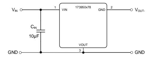
It is important to be aware that in this configuration the 173950x78 must withstand the sum of the input voltage and the absolute value of the output voltage ( $V_{IN} + |V_{OUT}|$ ), instead of just the input voltage. This means that the maximum operating voltage should be limited to  $28V - |V_{OUT}|$  (e.g. if the 173950578 is used in this configuration, the input voltage should not exceed 23V).
