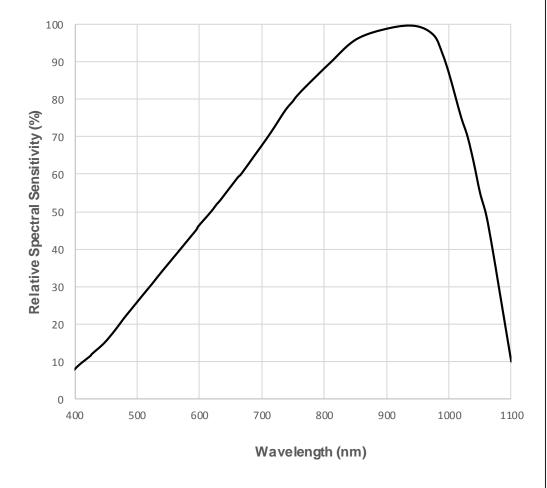
Testcondition: Ee=0,5mW/cm<sup>2</sup>; VCE=5V
