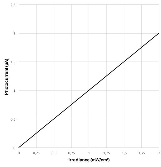
Testcondition: Ee= 0,5 mW/ cm<sup>2</sup>; VR=5V
