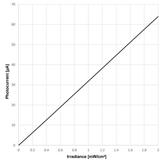
Testcondition: Ee=0,5 mW/cm<sup>2</sup>; VR=5V
