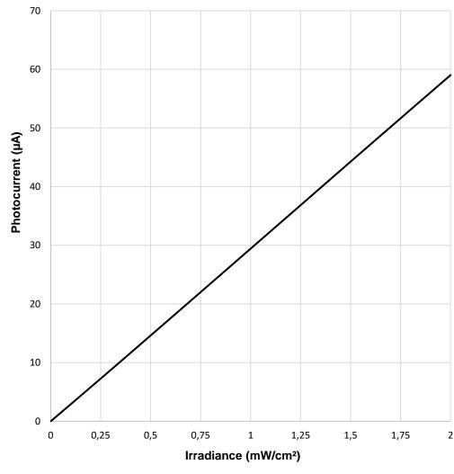
Testcondition: Ee= 0,5 mW/ cm<sup>2</sup>, VR=5V
