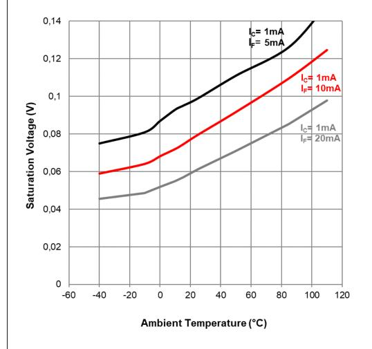
Testcondition: I<sub>E</sub>= 5mA, Normalized to 25°C
