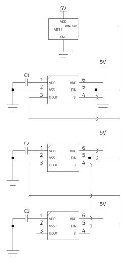
The information of each LED is transmitted with Most Significant Bit (MSB) first.
