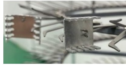
Figure 11: Anodization attachment example for stamped parts.
