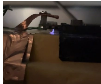
Figure 25: The gas discharge tube (GDT) passes a burst coupled with a capacitive coupling clamp to the SPoE interface which is operated with an unshielded twisted-pair cable.
