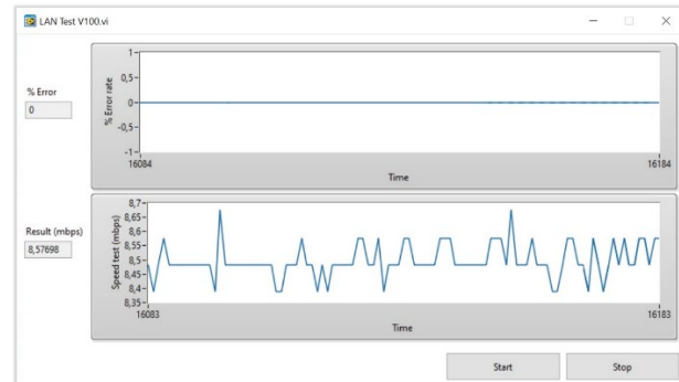
Figure 3: Monitoring the SPoE interface. PSE and PD are integrated into the network via an Ethernet interface.
