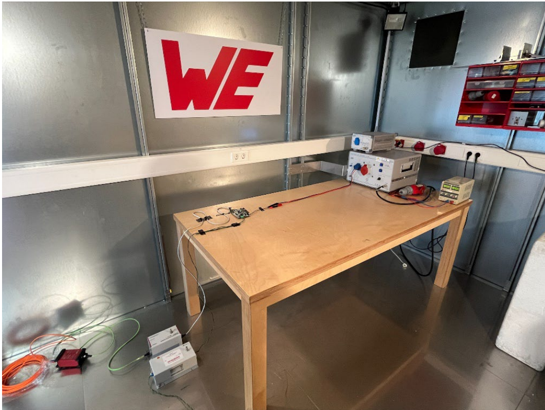
Figure 10: Measurement of conducted emissions at the PSE board of the SPoE reference design.
