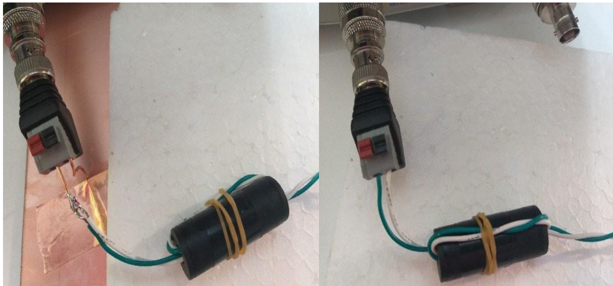
Figure 19: Configurations for the measurements. Left CM, i.e. wire 'a' and wire 'b' together against a ground plane on which the 2 m long twisted pair wire is positioned. Right DM, wire 'a' against wire 'b', without ground reference
