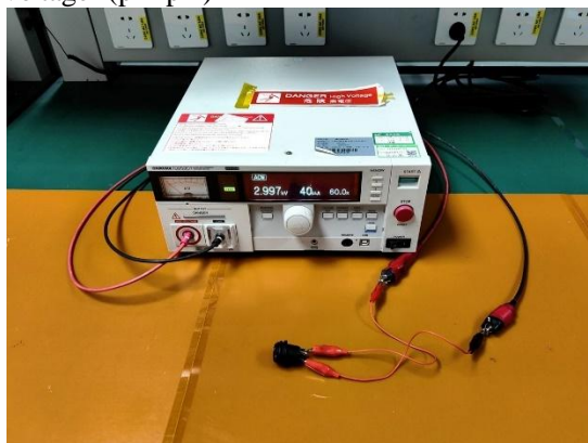
耐电压 Withstand voltage (pin-case)
