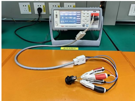
接触电阻 Contact Resistance
