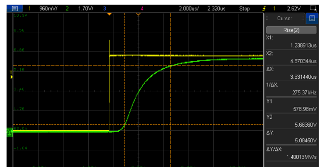
Figure 28: Turn-on example (WL-OCPT 817 Bin B) ( V_{RF} , V_{RC} )
