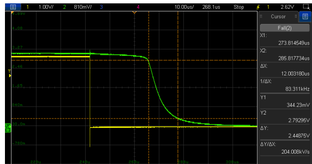
Figure 32: Turn-off transition (Bin D, V_{CE\_on} = 0.2 V) ( V_{RF} , V_{RC} )
