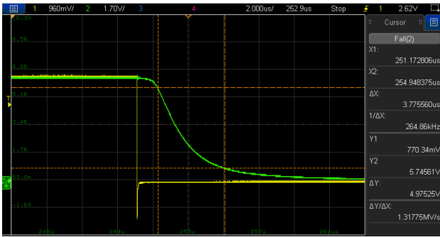
Figure 29: Turn-off example (WL-OCPT 817 Bin B) ( V_{RF} , V_{RC} )
