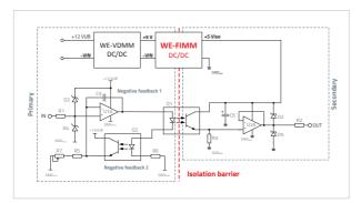
The application circuit of a galvanic isolated measurement signal transmission can provide a solution for decoupling by galvanic isolation and balancing of the measured values.
