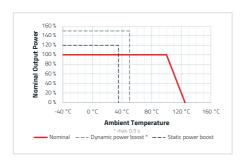
With the **power boost feature** additional current could be provided allowing the module to fulfil the demands in:
