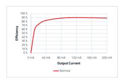
Due to its high **efficiency of up to 91%** it supports a "cool design" and can therefore be used in an operating temperature range from -40 °C up to 100 °C without any derating.
