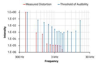
Figure 1: Measured voltage-signal frequency spectrum of 470µF aluminum electrolytic capacitor (WCAP-ASLI, 865080253012) at fundamental frequency of 448.9 Hz. Also shown, is the threshold of audible distortions as determined in psychoacoustic experiments for a fundamental at 500 Hz.
