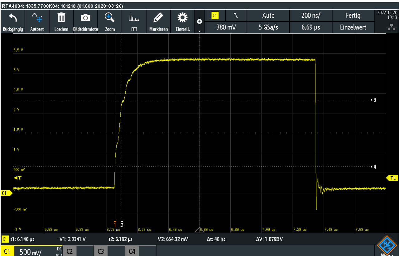
Figure 8: Reference measurement with 1 kΩ pull-ups + multilayer SMT ferrite + TVS diode array + 20 cm cable (= 46 ns rise time)
