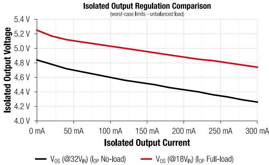
Figure 18: Voltage Regulation worst-case limits (unbalanced load)
