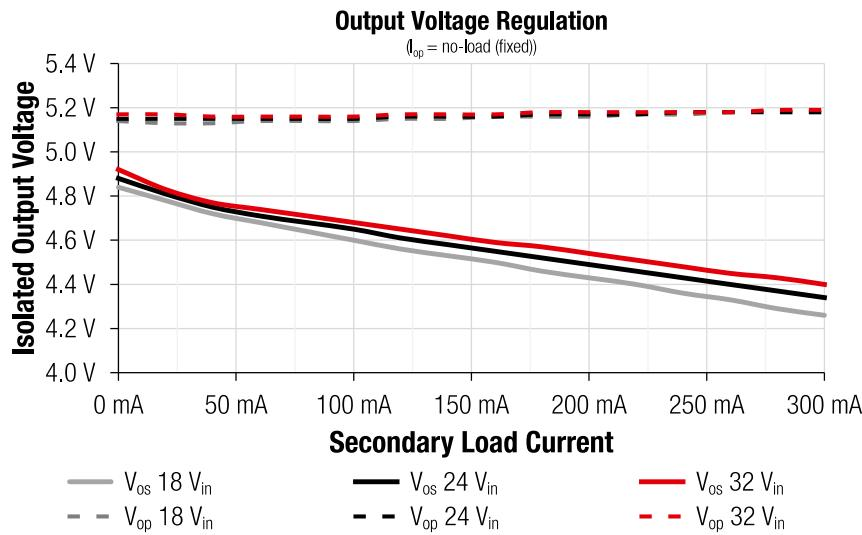
Figure 15: Voltage Regulation (at fixed  $I_{op}$  = no-load (unbalanced load))
