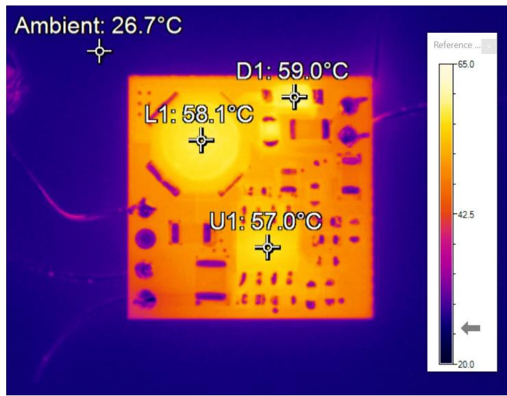
Figure 37: Board components temperature at  $V_{in}$  (nom) = 24 V and 25 °C ambient
