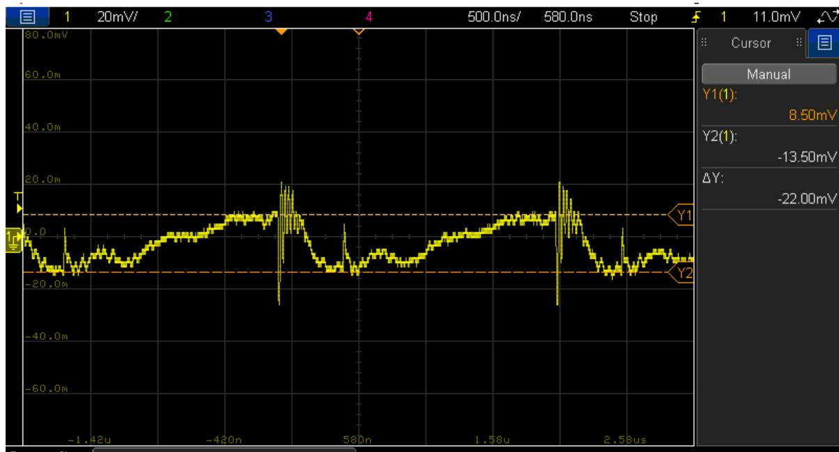
Figure 29: Secondary output voltage ripple (@  $V_{in} = 24$  V,  $I_{op} = I_{os} = 300$  mA (balanced full-load))
