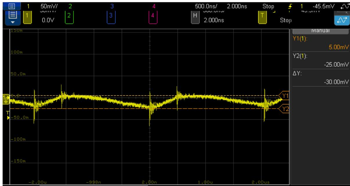
Figure 28: Primary output voltage ripple (@  $V_{in} = 24$  V,  $I_{op} = I_{os} = 300$  mA (balanced full-load))
