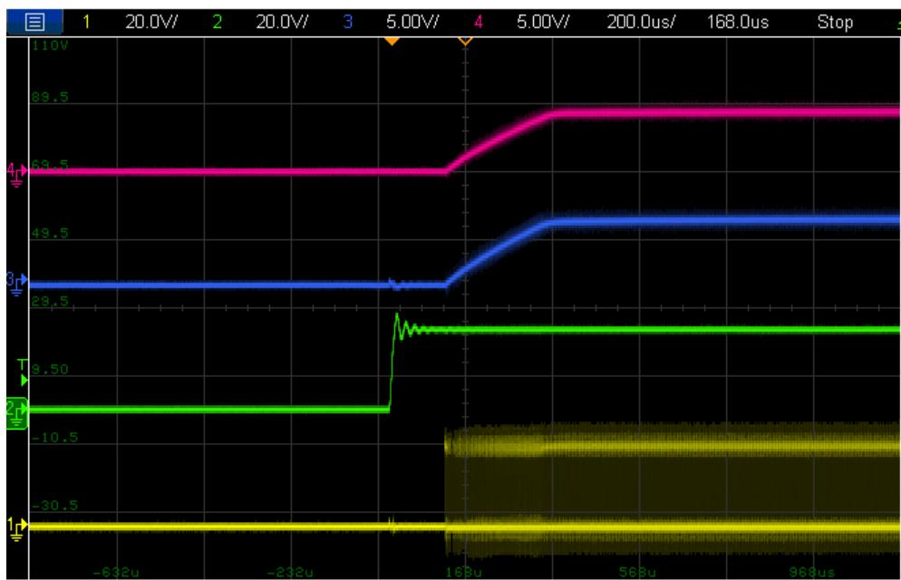
Figure 24: Start-up characteristic ( $V_{in} = 24\text{ V}$ ,  $I_{op} = I_{os} = 300\text{ mA}$  (full-load, balanced)) ( $V_{os}$ ,  $V_{op}$ ,  $V_{in}$ ,  $V_{sw}$ )
