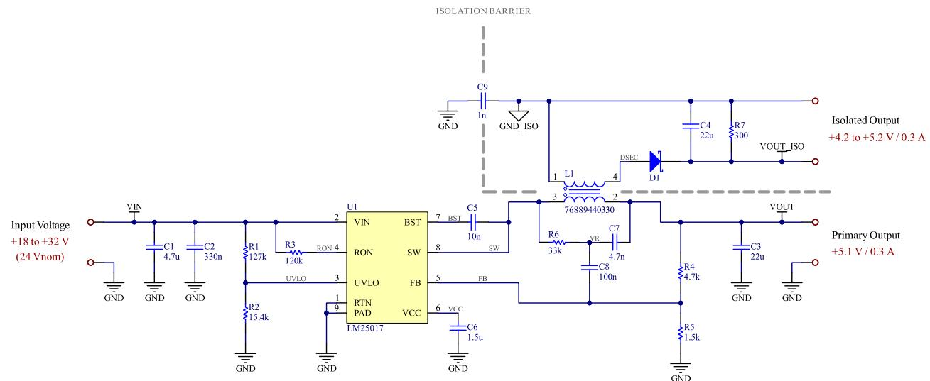
Figure 8: RD006 Schematic
