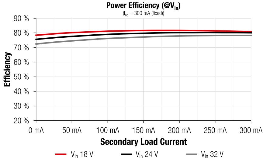
Figure 20: Power Efficiency (at fixed I<sub>op</sub> = 300 mA (unbalanced load))
