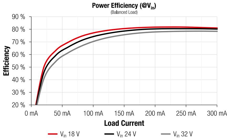
Figure 19: Power Efficiency (balanced load)
