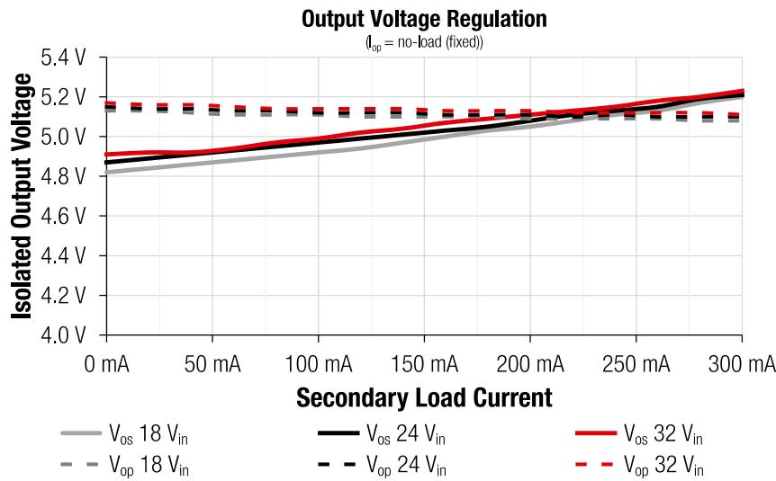
Figure 17: Voltage Regulation (at fixed  $I_{os} = \text{no-load}$  (unbalanced load))
