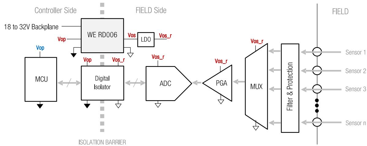
Figure 6: Multichannel PLC Analog Input Module example (simplified)
