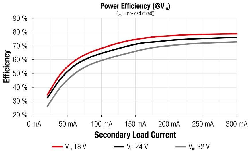
Figure 23: Power Efficiency (at fixed  $I_{os} = \text{no-load (unbalanced load)}$ )
