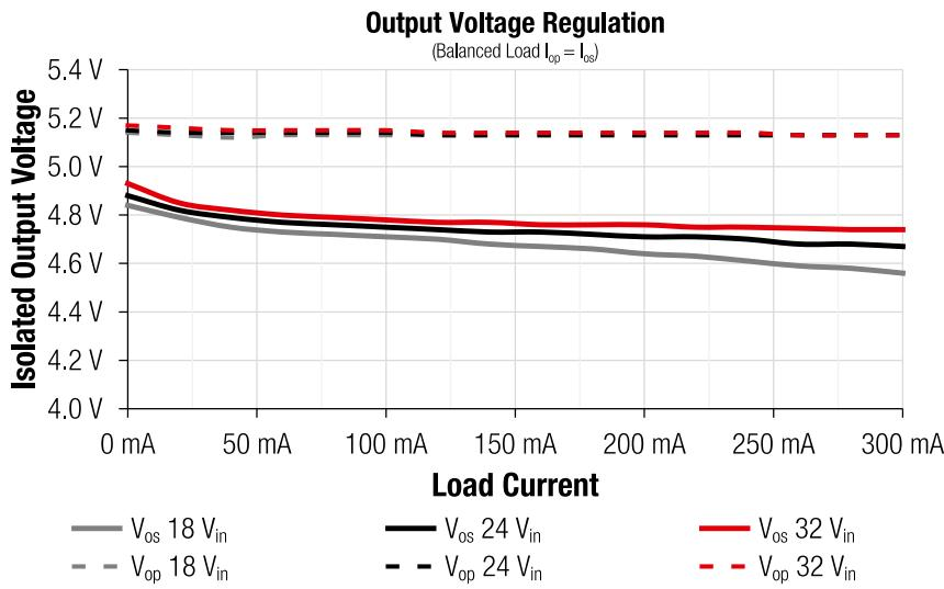
Figure 13: Voltage Regulation (at  $I_{op} = I_{os}$  (balanced load))
