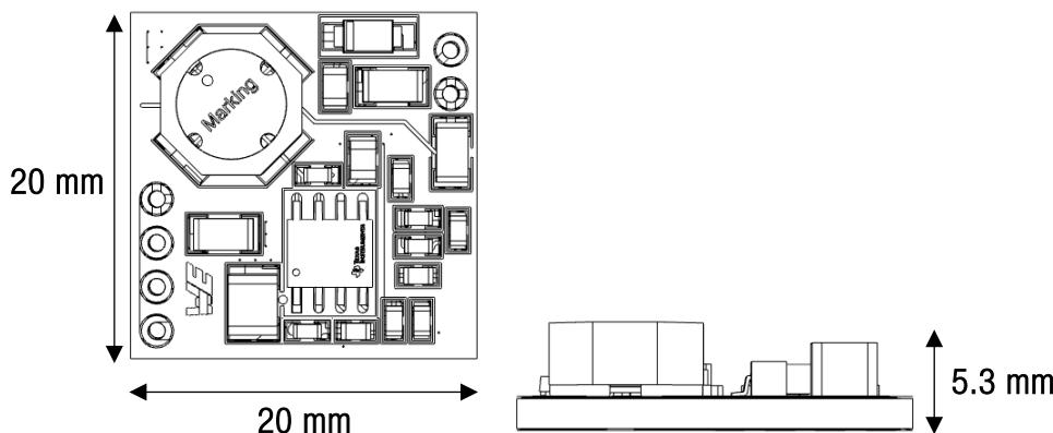
Figure 11: RD006 Board Dimensions: board sides (left), board height (with 1.5 mm thick PCB) (right)
