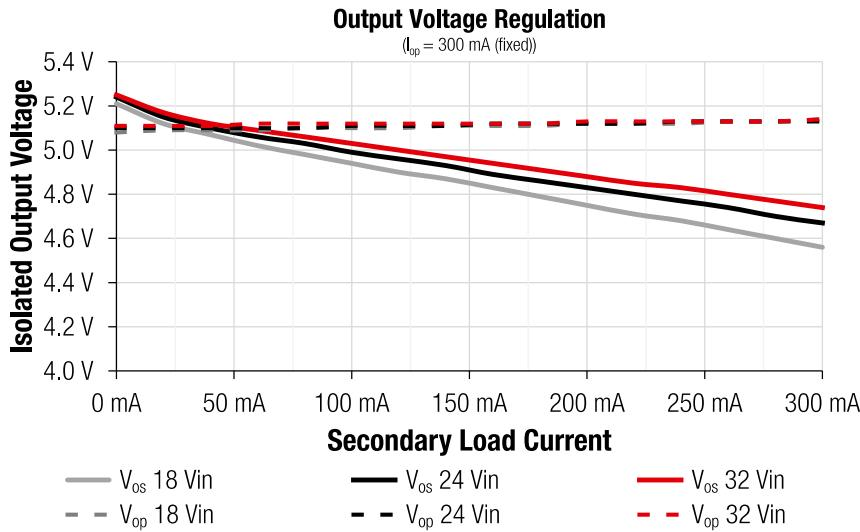
Figure 14: Voltage Regulation (at fixed  $I_{op} = 0.3$  A (unbalanced load))
