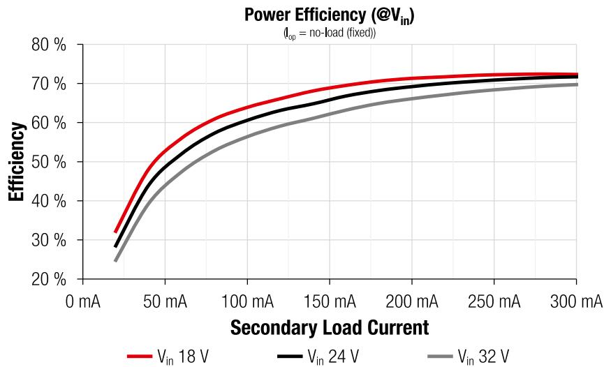
Figure 21: Power Efficiency (at fixed  $I_{op}$  = no-load (unbalanced load))
