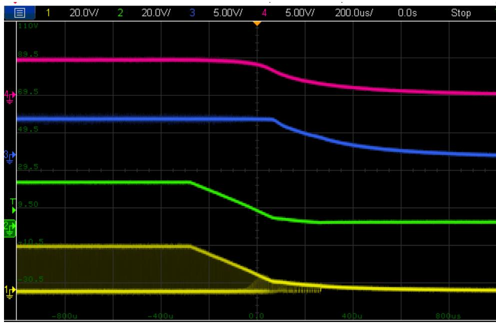
Figure 25: Shut-down characteristic ( $V_{in} = 24$  V,  $I_{op} = I_{os} = 300$  mA (full-load, balanced)) ( $V_{os}$ ,  $V_{op}$ ,  $V_{in}$ ,  $V_{sw}$ )
