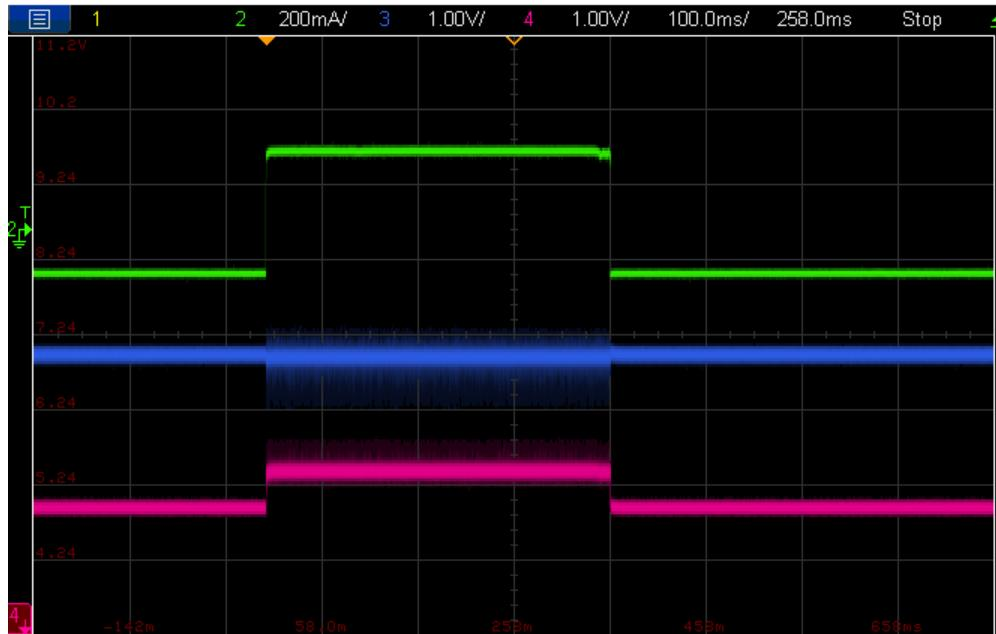
Figure 30: Load transient ( $I_{os}$  = no-load, Primary load current step 0 to 300 mA, 1 A/ $\mu$ s) ( $V_{os}$ ,  $V_{op}$ ,  $V_{in}$ )
