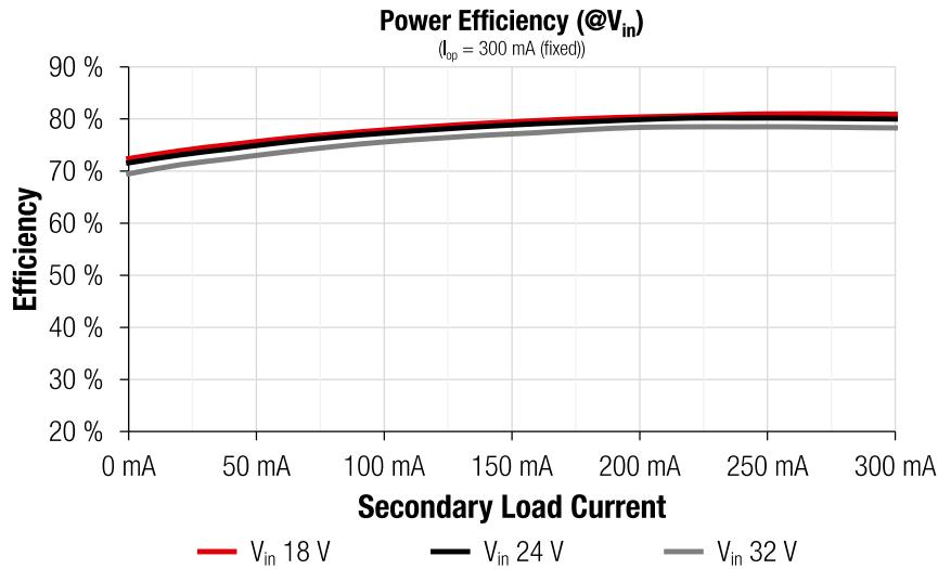
Figure 22: Power Efficiency (at fixed  $I_{os}$  = 300 mA (unbalanced load))
