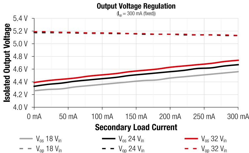
Figure 16: Voltage Regulation (at fixed  $I_{os}$  = 300 mA (unbalanced load))
