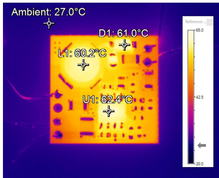
Figure 36: Board components temperature at  $V_{in}$  (max) = 32 V (worst-case) and 25 °C ambient
