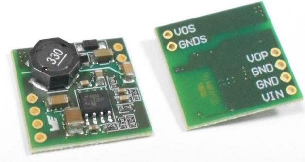
Figure 1: Board Image (top and bottom sides)
