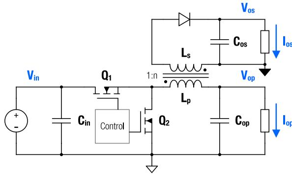
Figure 3: Buck Converter with Isolated Output Power Stage
