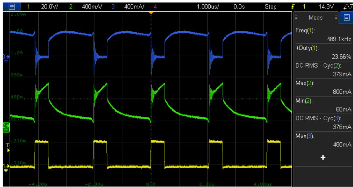
Figure 26: Winding currents and SW node voltage (@  $V_{in} = 24$  V,  $I_{op} = I_{os} = 300$  mA (balanced full-load)) ( $I_{os}$ ,  $I_{op}$ ,  $V_{sw}$ )
