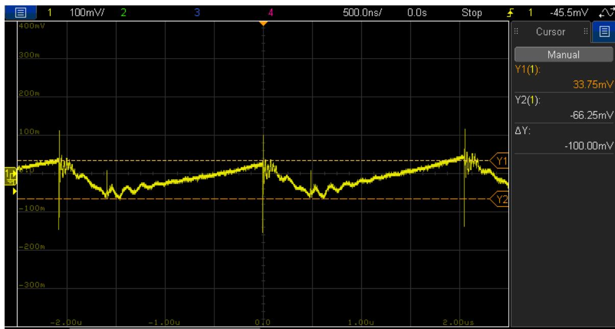
Figure 27: Input voltage ripple (@  $V_{in} = 24$  V,  $I_{op} = I_{os} = 300$  mA (balanced full-load))
