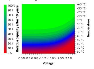
Figure 2: Contour plot shows the relative capacitance after 10 years for parameter sets of voltage (x-axes) and temperature (y-axes). The values of relative capacitance are encoded in the colour.
