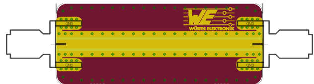
Figure 8: PCB layout top layer utilizing the via fence.
