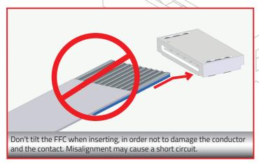
Insert the FFC horizontally until the conductor almost disappears. The conductor must hit the end of the FPC housing.
