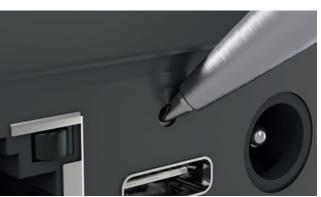
Special design of the push buttons' actuator tip (caved design) provides a perfect fix point for pen or other sharp tools while operation
