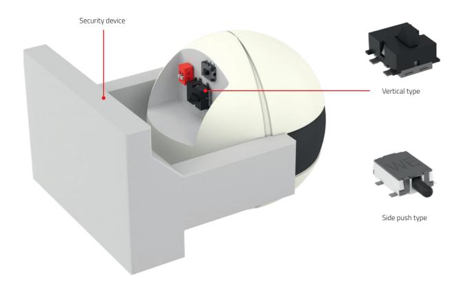
Tamper detection is the ability of a device to sense an active attack to the device and the threat of the attack should initiate an event (e.g. alarm, shutdown of the device).
