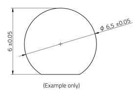
**Step 2.** Install connector through the opening panel cutout from the inside Be aware of maximum panel thickness recommended on datasheet
