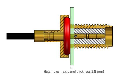
**Step 3.** Slide and twist the lock washer and hex nut onto connector body Tighten the hex nut to 57 N-cm using torque wrench to ensure IP67 rating
