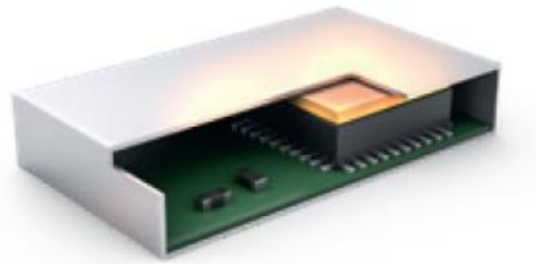
Figure 3: Functionality of a gap filler on an IC.
