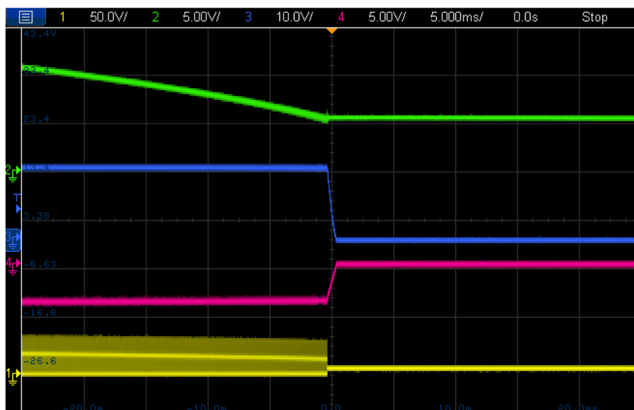
Figure 21: Shut-down at full-load
