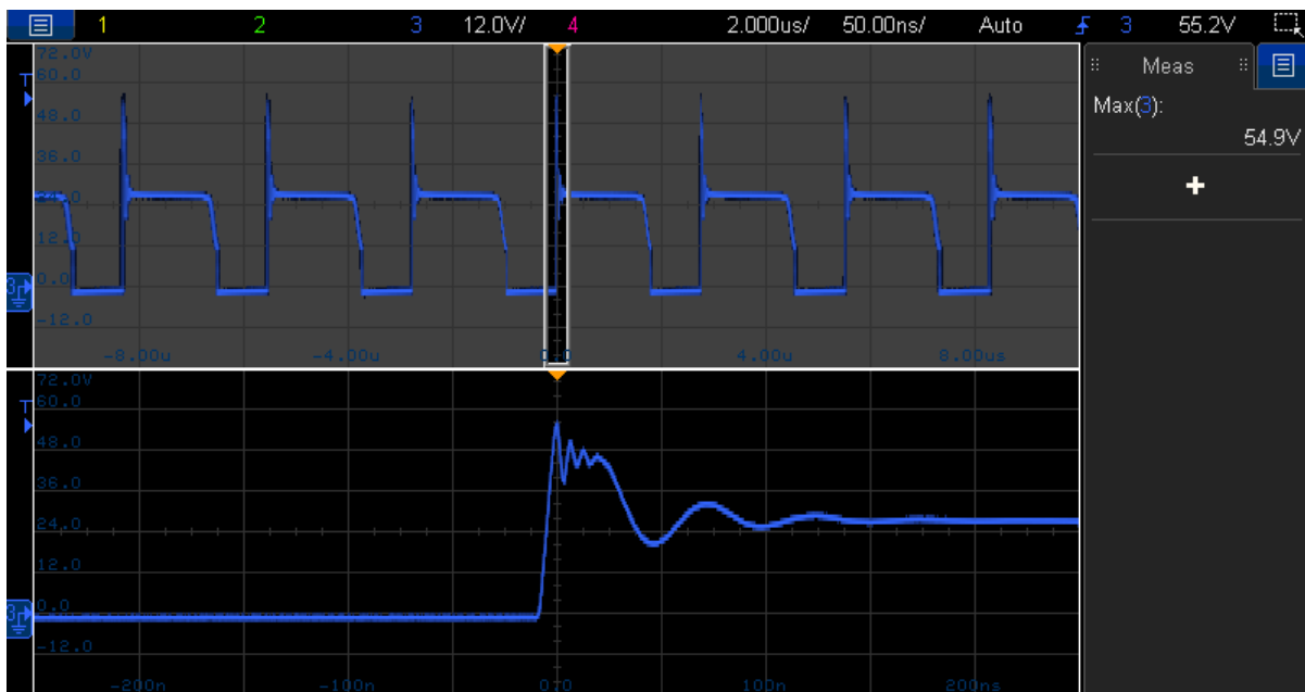
Figure 24: SW Node voltage clamping ( V_{in} = 18\text{ V} , P = 6\text{ W} )
