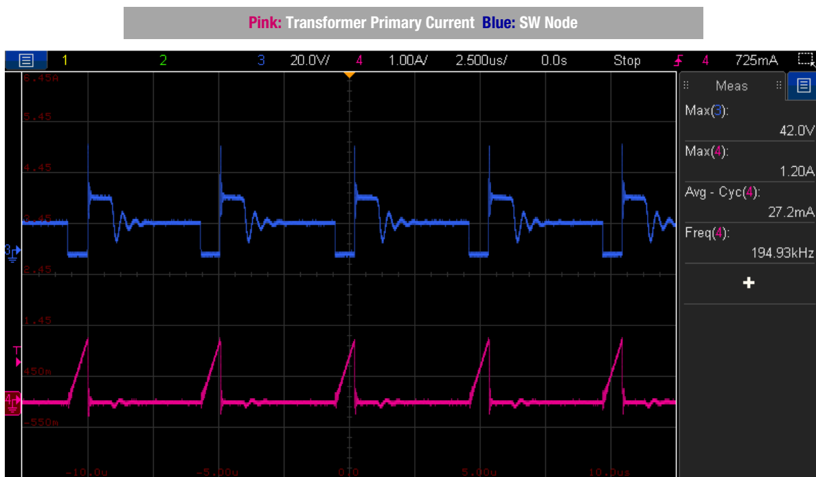
Figure 22: 1 W load (DCM operation)
