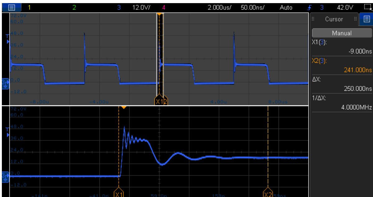
Figure 25: SW Node ringing damping ( V_{in} = 9\text{ V} , P = 6\text{ W} )
