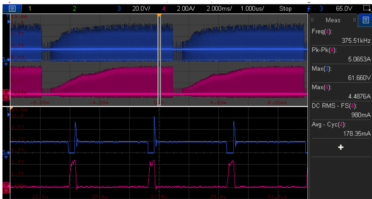
Figure 29: Short-circuit protection at V in = 18 V
