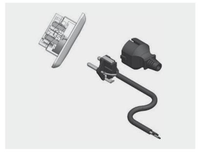
Fig. 1.2: Components of a wall plug/receptacle connector
